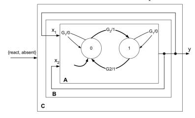
Q3.2 (20 points) Consider the finite-state machine composition shown below:
