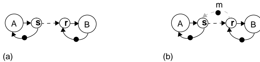
Figure 5.3. An IPC graph with a feedforward edge: (a) original graph (b) imposing bounded buffers.
