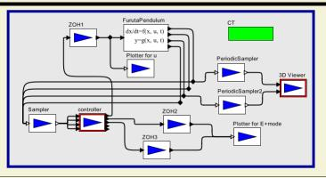
Ptolemy II model of an embedded control system and the system being controlled. This is a hierarchical, heterogeneous model that combines four models of computation.
