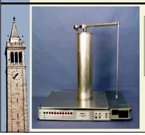
The Furuta pendulum has a motor controlling the angle of an arm, from which a free-swinging pendulum hangs. The objective is to swing the pendulum up and then balance it.
