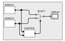
Figure 2: A variant of the program in figure 1 where the CONTROL process analyzes the data from the SOURCE processes before deciding how to merge them.
