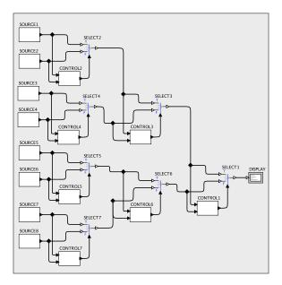
Figure 4: A variant of the program in figure 2 that merges 8 sources rather than two.
