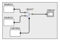
Figure 1: A simple five-process program, where messages from two SOURCE processes are merged based on messages from the CONTROL process and displayed by the DISPLAY process.
