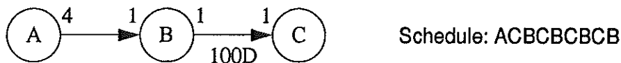
Fig 20. An example showing the benefits of decomposing the dynamic buffer component into a separate segment for each dynamic transaction.
