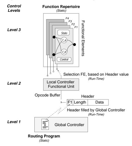
Figure 7.6. Control Hierarchy in the stream-based dataflow architecture.
