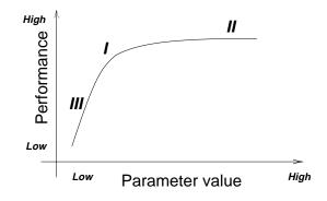
**Figure 1.5**. The relationship between a measured performance in the architecture and a range of parameter values. Point I indicates the best trade-off between a particular performance and parameter values. Point II shows a marginal increase of the performance at a large cost and point III shows a deterioration of the performance.
