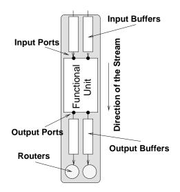
Figure 2.4. A processing element consists of a number of input and output *buffers*, a number of *routers* and one *functional unit*.
