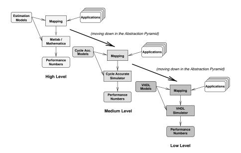
Figure 3.4. A stack of Y-chart environments, with a different model at each level of abstraction.
