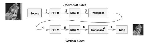
Figure B.1. The Picture in Picture Application
