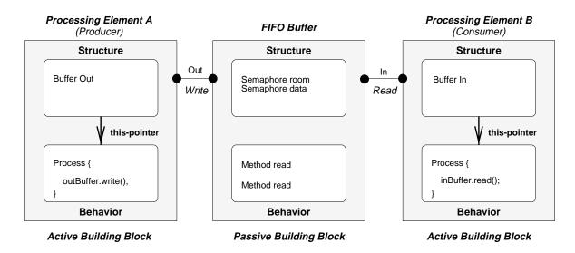
Figure 5.6. The producer/consumer system, revised to included building blocks to model the system.
