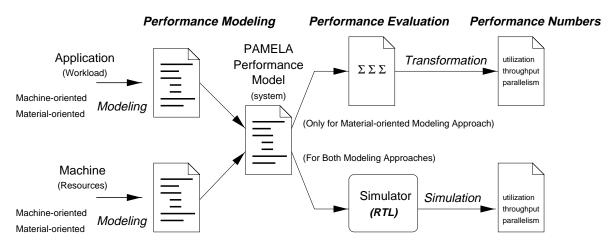
Figure 4.3. The two different objectives possible in performance analysis: ease of modeling versus ease of evaluation.
