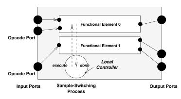
Figure 5.8. Model of a sample-switching FU.
