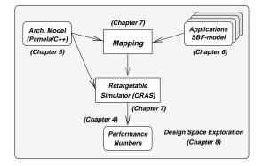
**Figure 3.7**. The Y-chart environment as we will build it in this thesis. The six main components (including the design space exploration) of the Y-chart environment are labeled with the number of the chapter containing the detailed discussion of the components.
