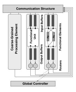
**Figure 2.2**. A detailed representation of the structure of a stream-based dataflow architecture. The architecture consists of a set of *processing elements*, a *communication structure*, and a *global controller*.
