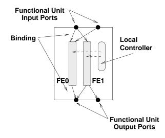
Figure 2.5. A functional unit consists of a set of *functional elements* (FE), a *local controller*, and input and output ports.
