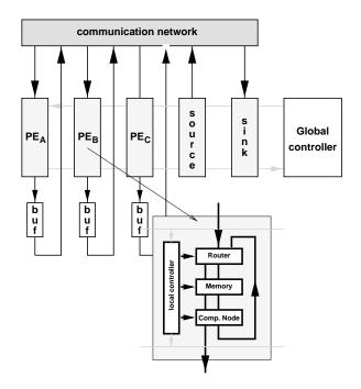
Figure 9.8. The architecture of the Jacobium processor.
