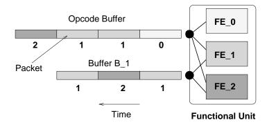
Figure 2.12. A functional unit in packet-switching mode that deadlocks due to a matching problem.
