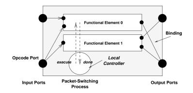
Figure 5.7. Model of a Packet-Switching FU.
