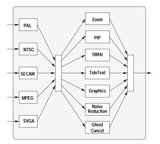
Figure 1.2. Video signal processing section of a modern high-end TV-set.
