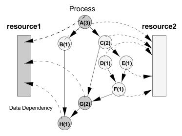
**Figure 4.2**. A simple system, composed of two resources (resource1 and resource2) and a workload described by a collection of tasks (A to H). The directed lines represent data dependencies governing the order in which tasks execute. The dashed lines indicate the resource a task must possess in order to execute.
