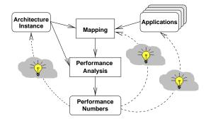
Figure 3.2. The Y-chart with lightbulbs indicating the three areas that influence performance of programmable architectures.
