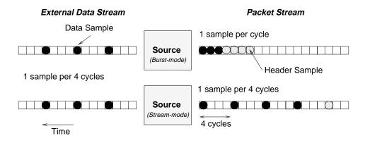
Figure 2.10. Two source functional units that operate on two external streams with a rate of 1 sample per 4 cycles.
