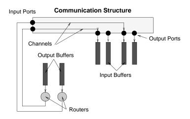
Figure 2.7. The communication structure.
