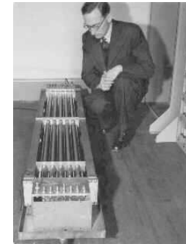
Mercury acoustic delay line. Used in the EDASC, 1947. 32 \times 17 bits
