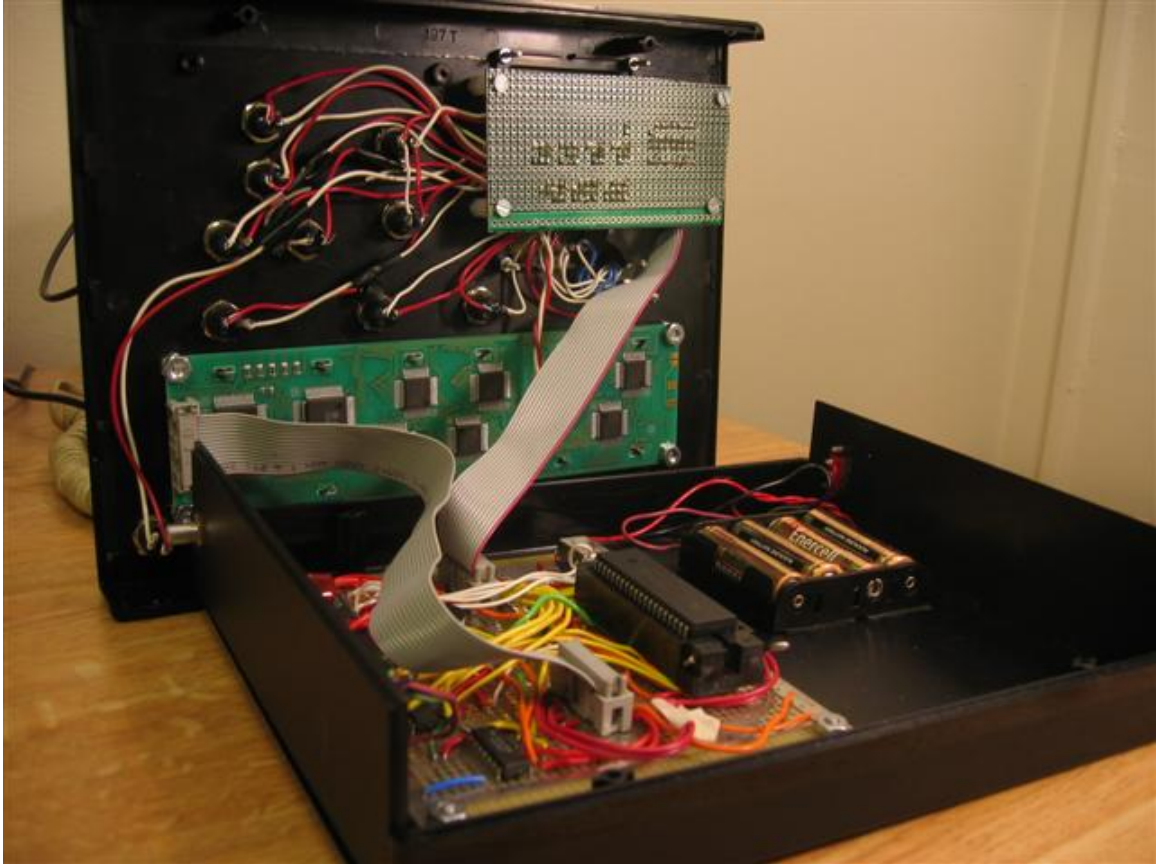
Figure 8: Internals of Machined Box Showing LCD, Dual PCBoards, Bus Ribbon Cables, and Battery Holder
