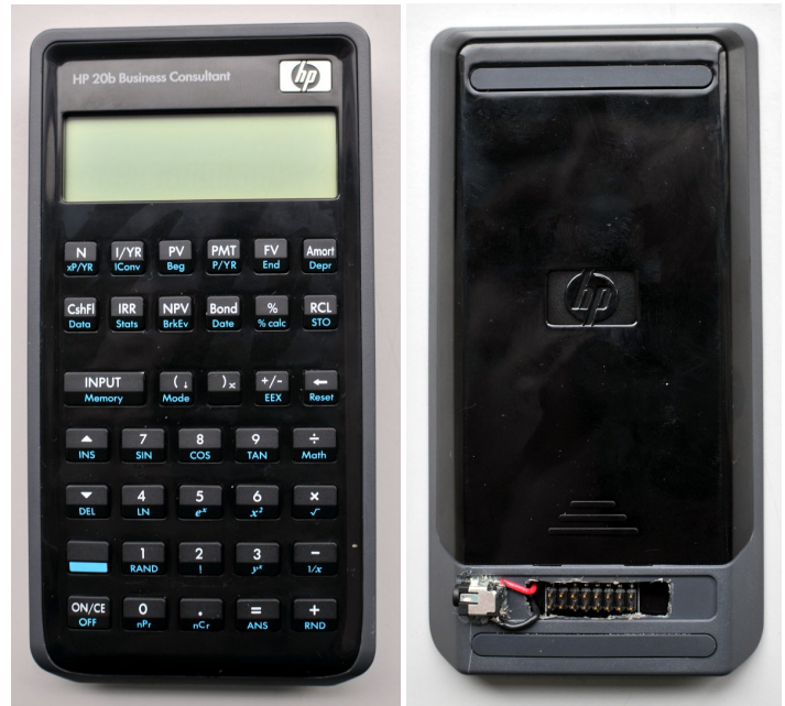
Figure 1: The front and back of the HP 20b calculator. I added the JTAG header and power connector so we could develop software on these without draining batteries.
