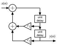
The triangular symbols represent systems where the output is simply the input scaled by a constant  $c_1$  or  $c_2$ .
