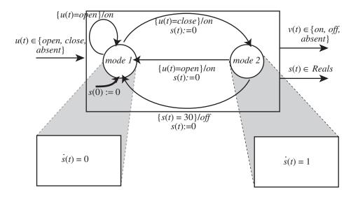
When someone opens the door (u(t) = open), the light is turned on (v(t) = on). After the door is closed (u(t) = close) for 30 seconds, the light is turned off (v(t) = off). Note that the door must be closed for the entire 30 seconds, before the light is turned off.
