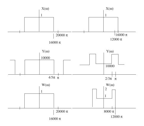
Figure 3: The graphs on the left are for T = 1/20000; the graphs on the right are for T = 1/12000.
