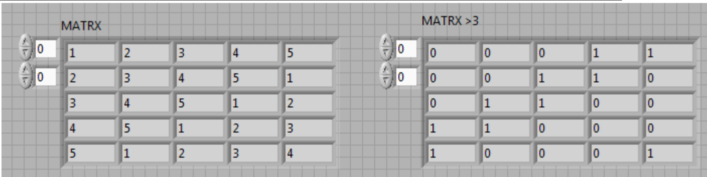
Figure 9 Thresholding: Example of how to use the greater than operator using a matrix and a scalar
