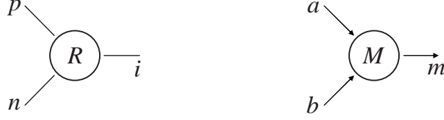
Figure 2.8. Graphical representation of processes. The process R on the left relates signals p , n , and i , R(p, n, i) . The process M on the right is functional with respect to I = (a, b) and O = (m) , m = M(a, b) .
